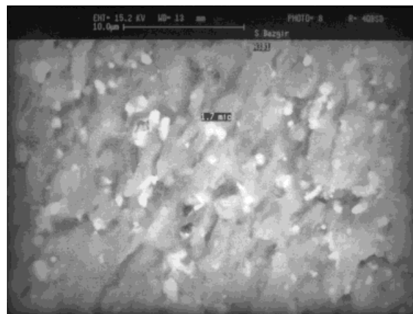
Figure 5 SEM micrograph of dynamically vulcanized 50/50 EPDM/PP blend loaded with 10 phr carbon black. Carbon black was added to the mix as an ingredient.
